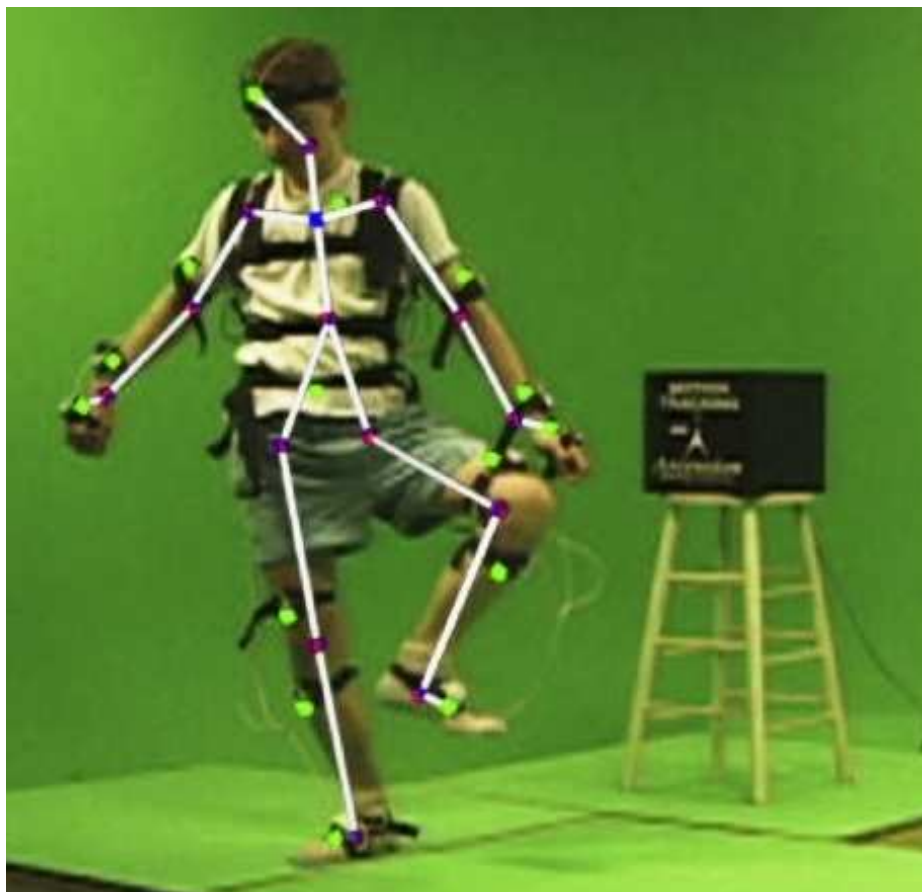
Figure 2.5: Test subject and generated model. The subject is wearing the motion capture equipment during a capture session; the superimposed skeletal model is generated automatically from the acquired motion capture data. The chest and pelvis sensors are located on the subjects back [4].
